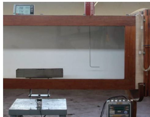
Figure 2. Train wagon model test in wind tunnel.
